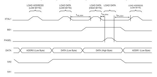
Note: 1. The timing requirements shown in Figure 29-7 (i.e., t<sub>DVXH</sub>, t<sub>XHXL</sub>, and t<sub>XLDX</sub>) also apply to loading operation.
