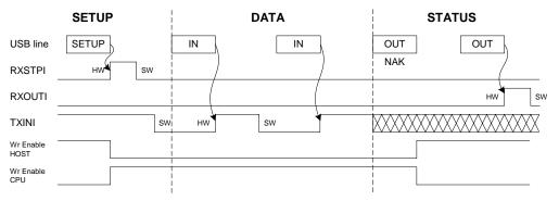
A NAK handshake is always generated at the first status stage command.
