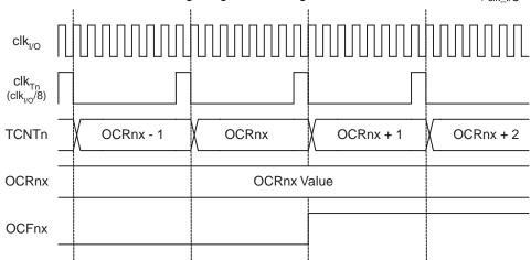
Figure 14-11. Timer/Counter Timing Diagram, Setting of OCFnx, with Prescaler (f<sub>clk I/O</sub>/8)
