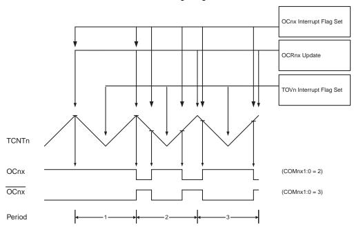
Figure 15-7. Phase Correct PWM Mode, Timing Diagram
