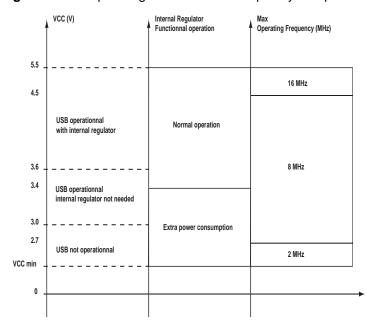
Figure 21-2. Operating modes versus frequency and power-supply
