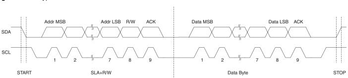
Figure 20-6. Typical Data Transmission
