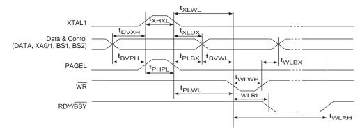
Figure 29-8. Parallel Programming Timing, Loading Sequence with Timing Requirements<sup>(1)</sup>
