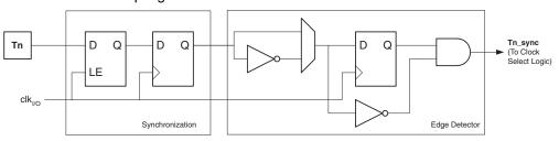
The synchronization and edge detector logic introduces a delay of 2.5 to 3.5 system clock cycles from an edge has been applied to the Tn pin to the counter is updated.
