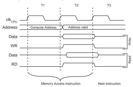
Figure 5-3. On-chip Data SRAM Access Cycles
