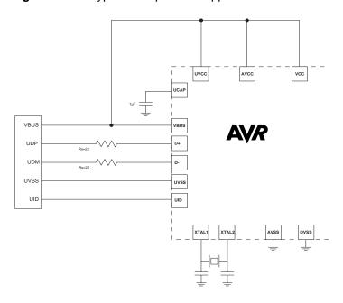
Figure 21-4. Typical Bus powered application with 3V I/O
