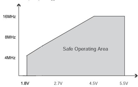
Figure 30-2. Maximum Frequency vs. V<sub>CC</sub>, AT90USB64/128
