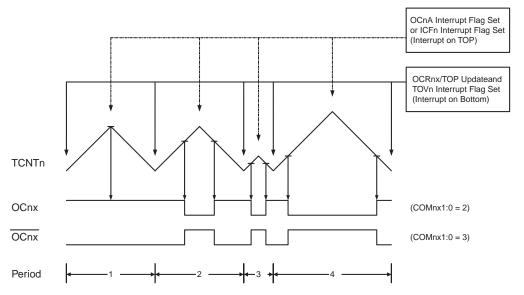
The Timer/Counter Overflow Flag (TOVn) is set at the same timer clock cycle as the OCRnx Registers are updated with the double buffer value (at BOTTOM). When either OCRnA or ICRn is used for defining the TOP value, the OCnA or ICFn Flag set when TCNTn has reached TOP. The Interrupt Flags can then be used to generate an interrupt each time the counter reaches the TOP or BOTTOM value.
