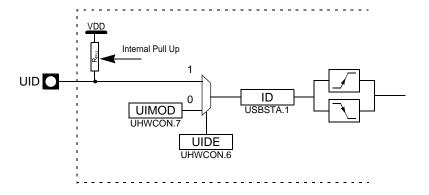
The ID pin can be used to detect the USB mode (Peripheral or Host) or software selected. This allows the UID pin to be used has general purpose I/O even when USB interface is enable. When the UID pin is selected, by default, (no A-plug or B-plug), the macro is in the Peripheral
