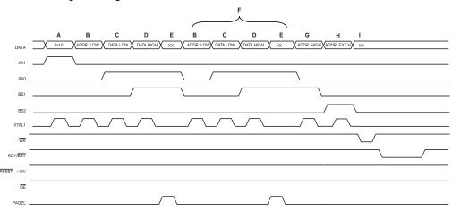
Figure 29-3. Programming the Flash Waveforms<sup>(1)</sup>
