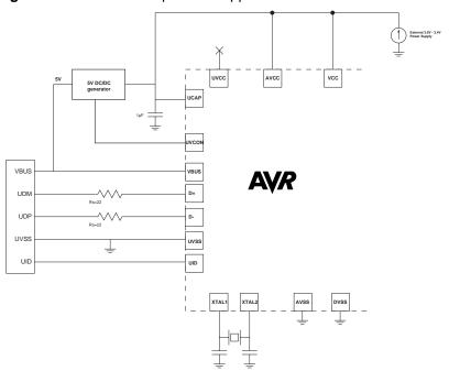
Figure 21-8. Host/OTG powered application with 5V I/O
