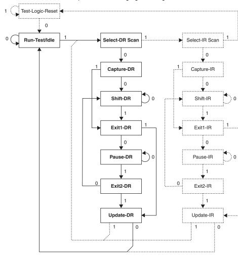
Figure 29-15. State Machine Sequence for Changing/Reading the Data Word
