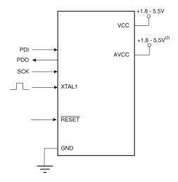
Notes: 1. If the device is clocked by the internal Oscillator, it is no need to connect a clock source to the XTAL1 pin.
