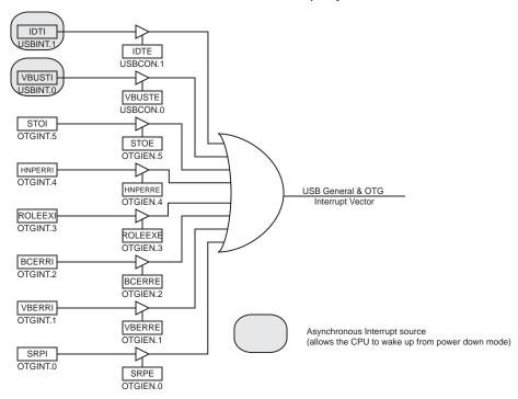
Figure 21-13. USB General and OTG Controller Interrupt System
