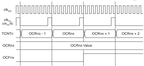
Figure 15-11 shows the setting of OCF2A and the clearing of TCNT2 in CTC mode.
