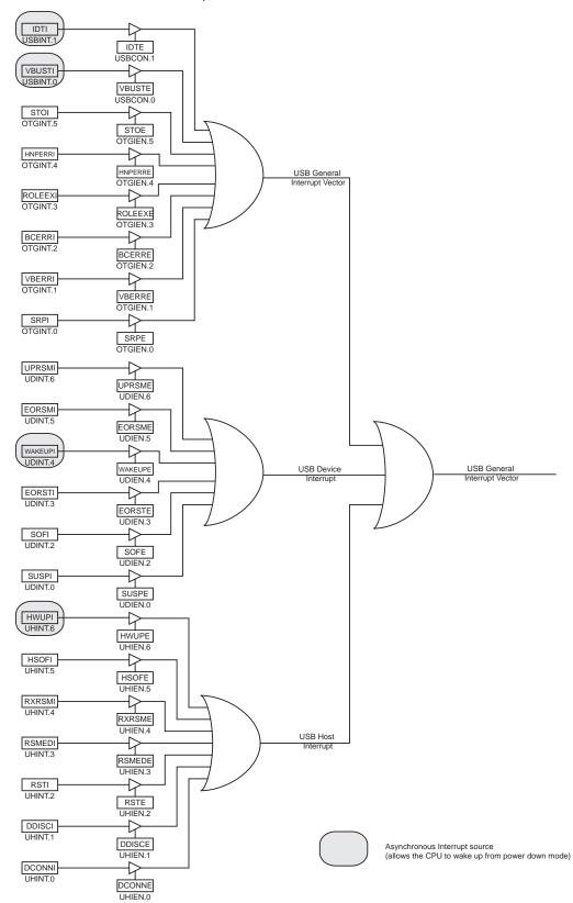
Figure 21-11. USB General interrupt vector sources
