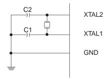
The Low Power Oscillator can operate in three different modes, each optimized for a specific frequency range. The operating mode is selected by the fuses CKSEL3..1 as shown in Table 6-3.
