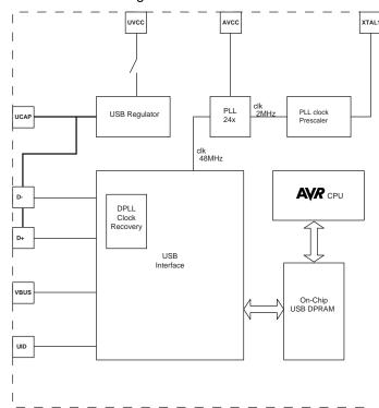
Figure 21-1. USB controller Block Diagram overview
