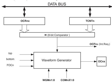
Figure 13-3. Output Compare Unit, Block Diagram
