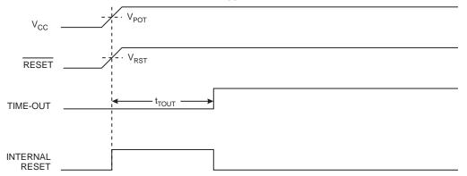
Figure 8-3. MCU Start-up, RESET Extended Externally
