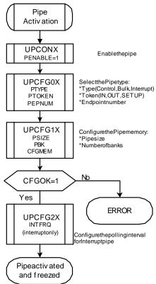
Once the Pipe is activated (EPEN set) and, the hardware is ready to send requests to the Device.
