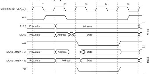
**Figure 5-7.** External Data Memory Cycles with SRWn1 = 0 and SRWn0 =  $1^{(1)}$
