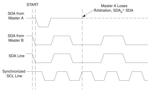
Figure 20-8. Arbitration Between Two Masters
