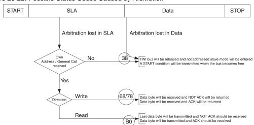
Figure 20-22. Possible Status Codes Caused by Arbitration
