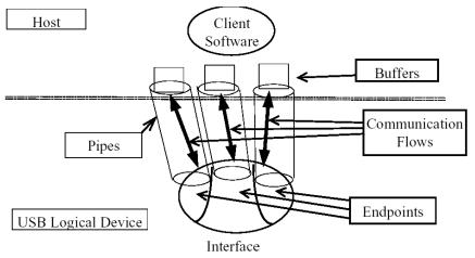
In the USB Host controller, a Pipe will be associated to a Device Endpoint, considering the Device Configuration Descriptors.
