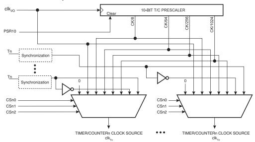
Figure 2. Prescaler for synchronous Timer/Counters
