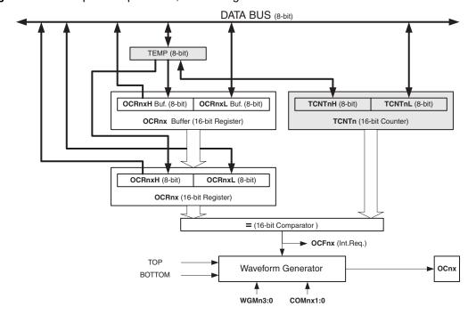
Figure 14-4. Output Compare Unit, Block Diagram
