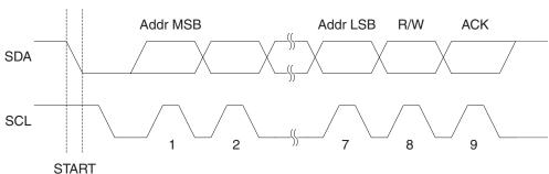
Figure 20-4. Address Packet Format
