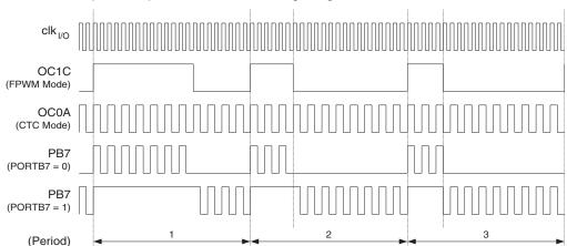
Figure 16-3. Output Compare Modulator, Timing Diagram
