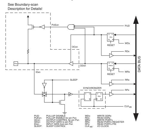
Figure 27-4. General Port Pin Schematic Diagram
