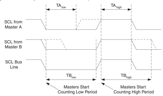
Figure 20-7. SCL Synchronization Between Multiple Masters
