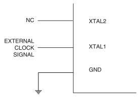
When this clock source is selected, start-up times are determined by the SUT Fuses as shown in Table 6-11.
