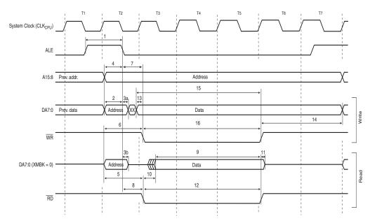
Figure 30-10. External Memory Timing (SRWn1 = 1, SRWn0 = 1)<sup>()</sup>
