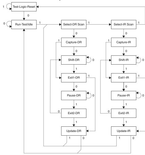
Figure 26-2. TAP Controller State Diagram
