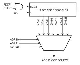
By default, the successive approximation circuitry requires an input clock frequency between 50 kHz and 200 kHz to get maximum resolution. If a lower resolution than 10 bits is needed, the input clock frequency to the ADC can be higher than 200 kHz to get a higher sample rate. Alternatively, setting the ADHSM bit in ADCSRB allows an increased ADC clock frequency at the expense of higher power consumption.
